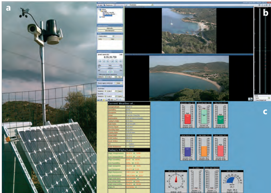
Figure 11 - Remote control system with Video-Meteo centre (a); acquisition software screen for video images (b); meteorological data acquisition software screen (c).
