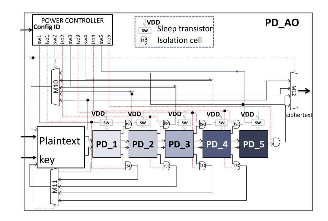
**Coarse Grained Reconfigurable AES** architecture capable of unrolling up to 10 rounds. Depending on the Configuration ID, the multiplexers change the connections among the RFs and RKs blocks, enabling different AES configurations.
