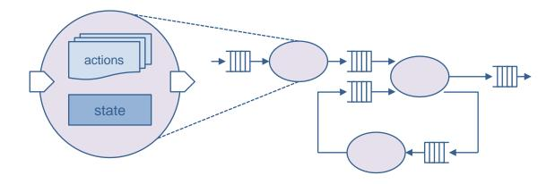
Actors encapsulate their state and communicate exclusively by sending and receiving tokens. Such an absence of race conditions, along with the intrinsic **modularity** of the dataflow graphs, make it possible to explicit the algorithmic **parallelism** of the programs.
