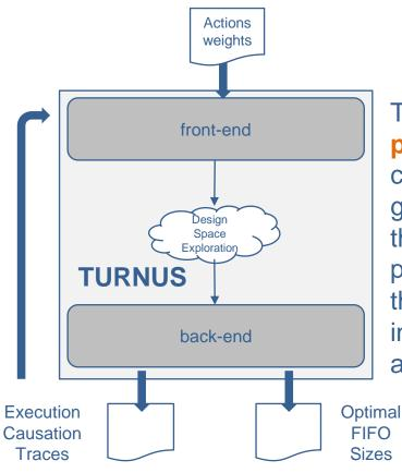
The causation traces postprocessing analyses the causation traces along with given action weights (latency of the actions for a specific target platform) in order to optimize the size of the FIFO memories in the dataflow network through a Design Space Exploration.
