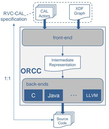
Open RVC-CAL Compiler (ORCC) is a framework able to generate, from an RVC-CAL specification, the corresponding source code for different target platforms (hardware, software or mixed).
