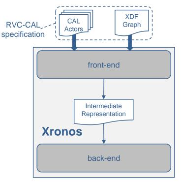
**Xronos** is a framework for the generation of RTL descriptions from dataflow or sequential applications. It supports three basic data types (int, uint and bool), flow control statements (branches, loops, parallel blocks) and procedural abstractions (sequences of statements) called *tasks*.
