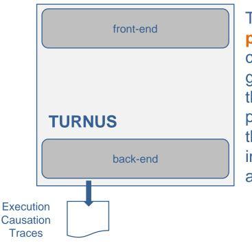
The causation traces postprocessing analyses the causation traces along with given action weights (latency of the actions for a specific target platform) in order to optimize the size of the FIFO memories in the dataflow network through a Design Space Exploration.
