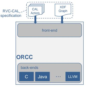
Open RVC-CAL Compiler (ORCC) is a framework able to generate, from an RVC-CAL specification, the corresponding source code for different target platforms (hardware, software or mixed).
