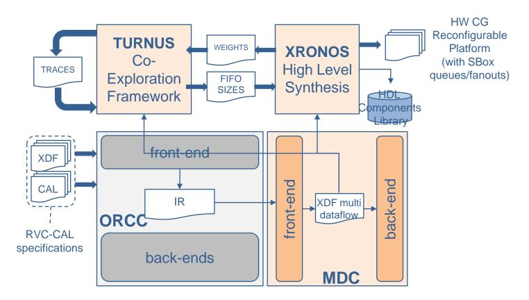
**STEP 4:** Xronos generates the RVC compliant reconfigurable hardware platform
