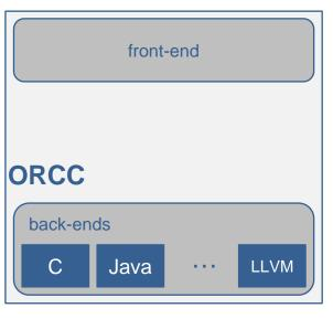
Open RVC-CAL Compiler (ORCC) is a framework able to generate, from an RVC-CAL specification, the corresponding source code for different target platforms (hardware, software or mixed).
