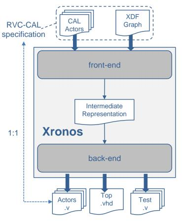
Xronos is a framework for the generation of RTL descriptions from dataflow or sequential applications. It supports three basic data types (int, uint and bool), flow control statements (branches, loops, parallel blocks) and procedural abstractions (sequences of statements) called *tasks*.
