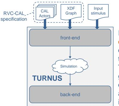
It provides the **execution causation traces** for a given dataflow specification in relation to a particular input stimulus. The causation traces are graphs describing the dependencies among the actions executed during the input stimulus processing.
