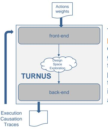
The causation traces postprocessing analyses the causation traces along with given action weights (latency of the actions for a specific target platform) in order to optimize the size of the FIFO memories in the dataflow network through a Design Space Exploration.
