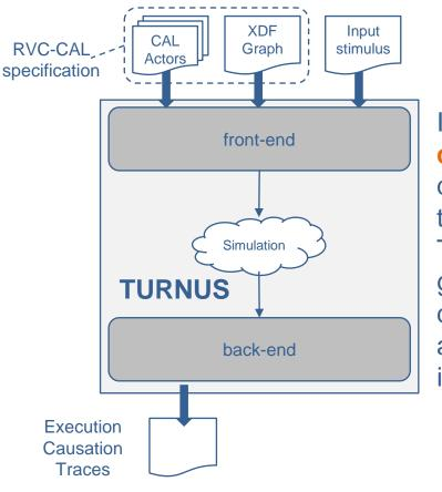
It provides the **execution causation traces** for a given dataflow specification in relation to a particular input stimulus. The causation traces are graphs describing the dependencies among the actions executed during the input stimulus processing.
